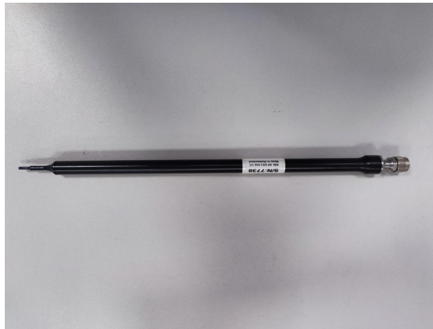
Figure 1-Speag COMOSAR Dosimetric E field Dipole
