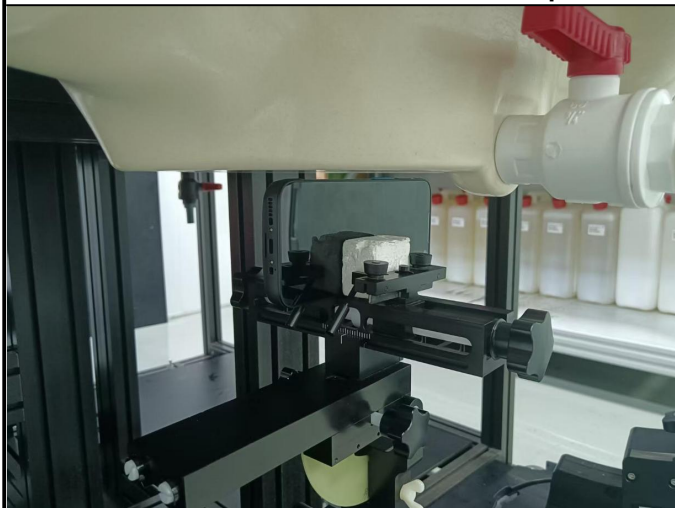
Left Side of EUT with 0.5 cm Gap
