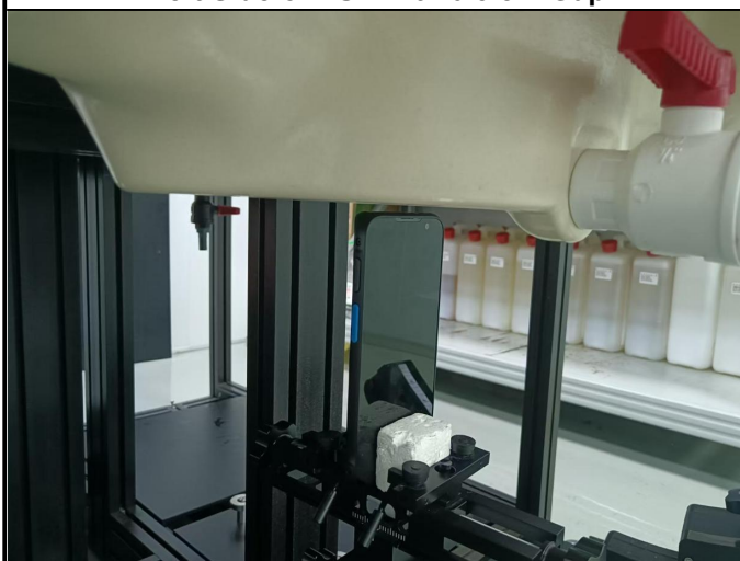
Top Side of EUT with 0.5 cm Gap
