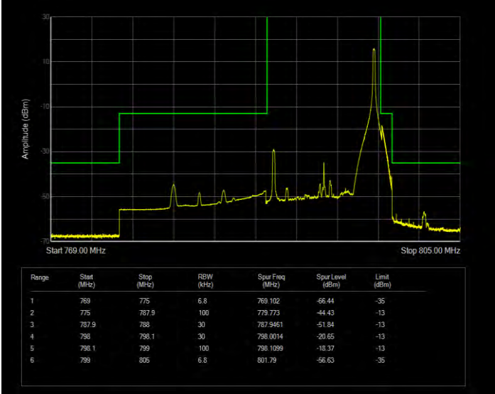
Band14 16QAM BW=10MHz Channel=23330 RB Size=50 Position=#0 Extended
