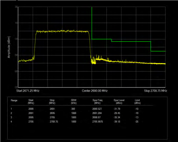
Band41 QPSK BW=15MHz Channel=41515 RB Size=75 Position=#0 Normal
