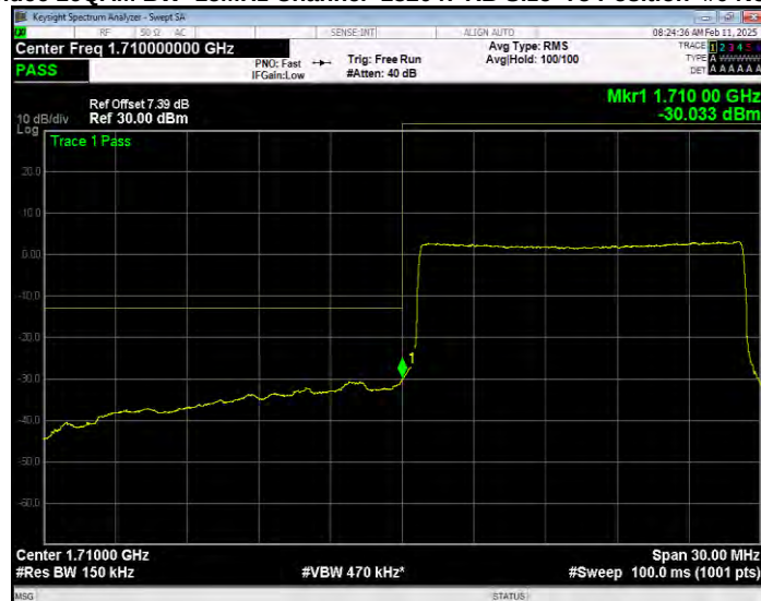
Band66 16QAM BW=15MHz Channel=132047 RB Size=75 Position=#0 Normal
