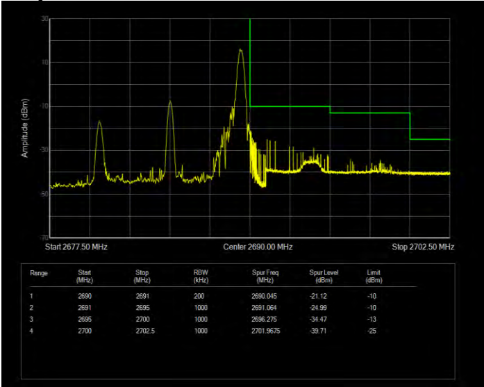
Band41 QPSK BW=10MHz Channel=41540 RB Size=50 Position=#0 Extended
