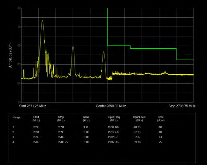
Band41 16QAM BW=15MHz Channel=41515 RB Size=1 Position=#Max Extended
