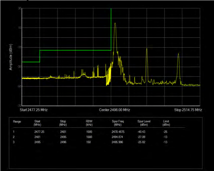
Band41 16QAM BW=15MHz Channel=39725 RB Size=1 Position=#Max Extended
