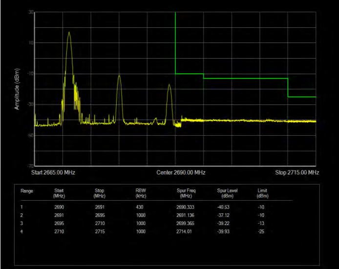
Band41 16QAM BW=20MHz Channel=41490 RB Size=1 Position=#Max Extended
