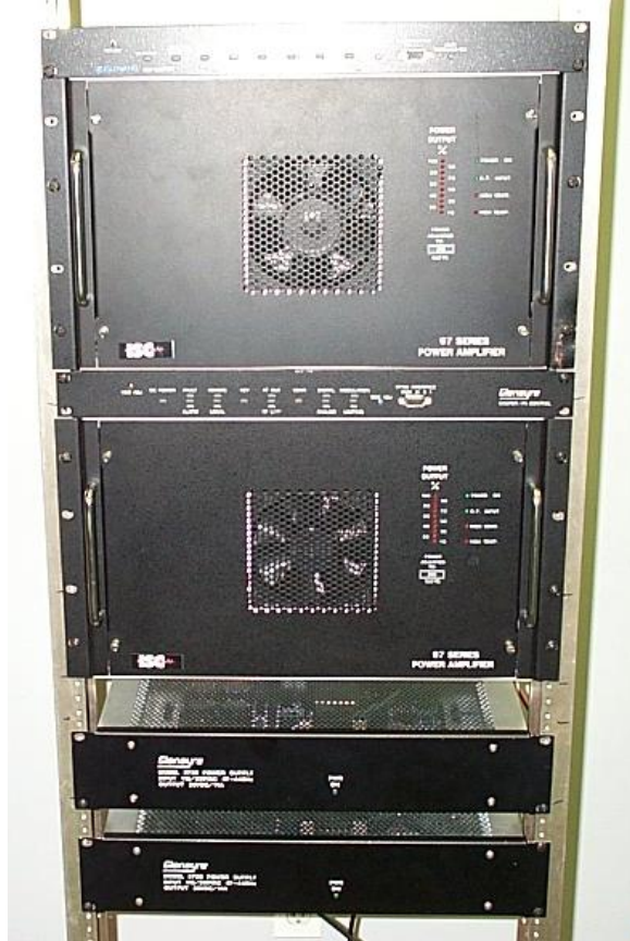
Front of EUT (2 amplifiers, 2 Exciters and 2 power supplies)
