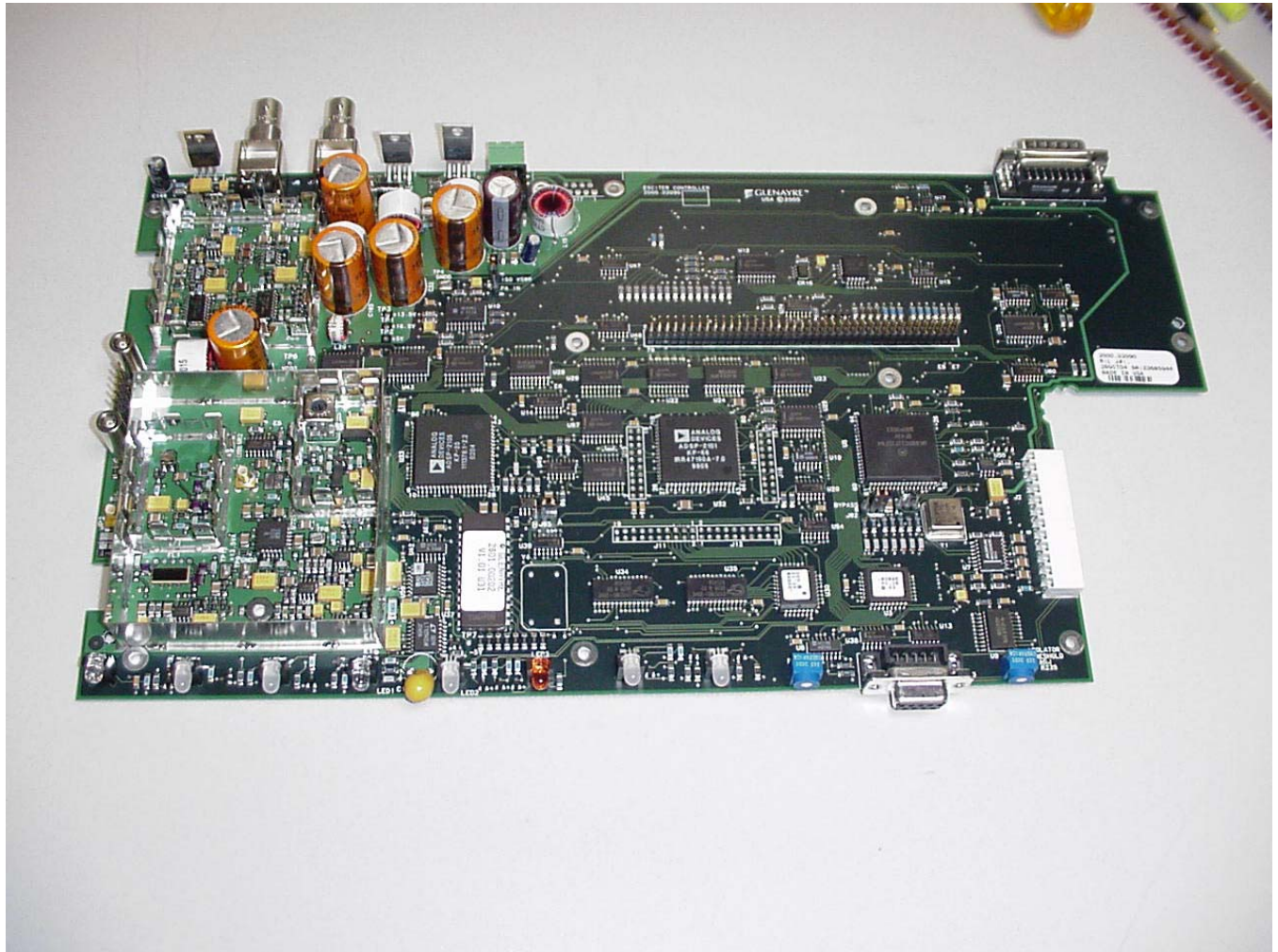
2000.02090 DSP Exciter Control Board (covers removed)
