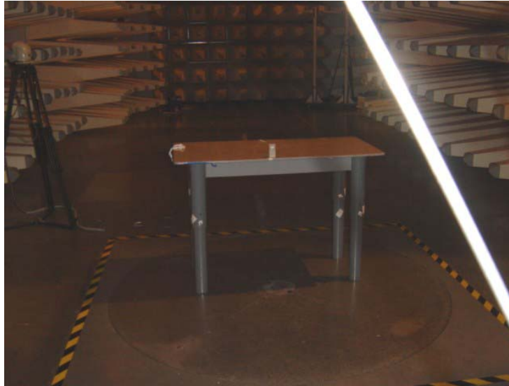
Set-up for Radiation Emission ( Transmitter)
