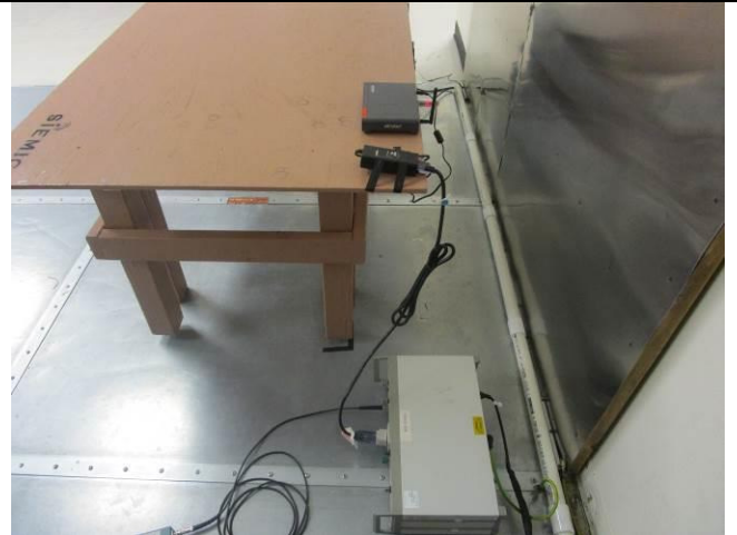
Conducted Emission Test setup – Rear View
