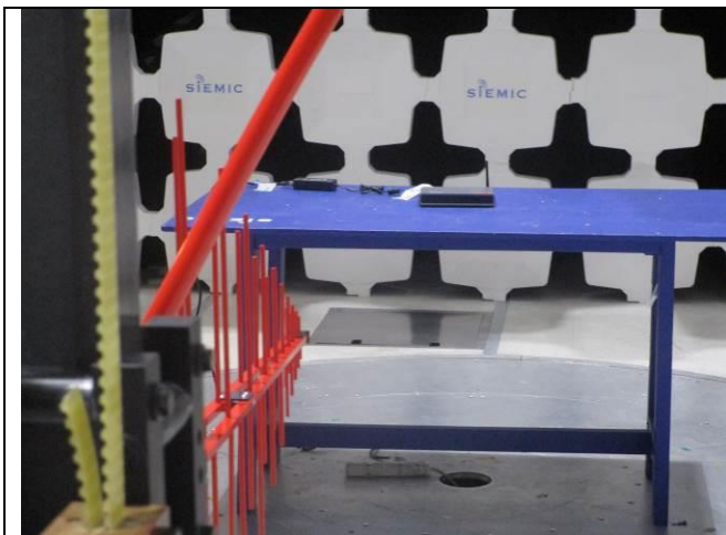
Radiated Emission Test setup (<1GHz) – Front View
