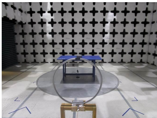
Radiation Emission Test setup (<30MHz) – Front View 0 deg
