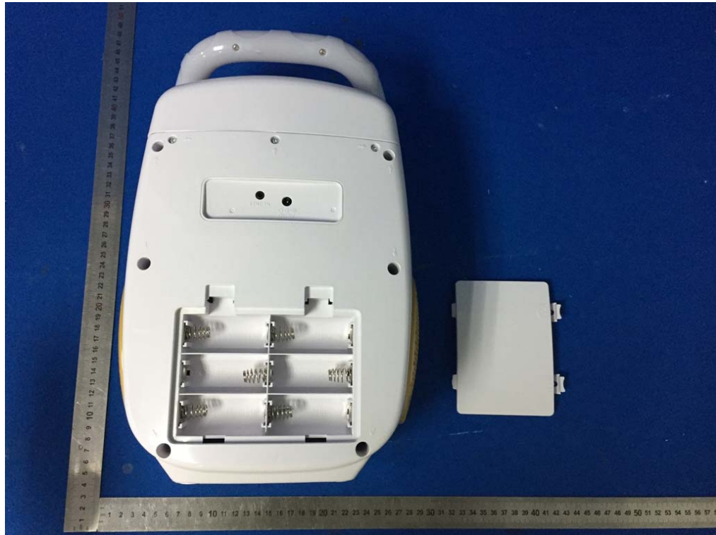
Fig. 9 Battery view of main unit
