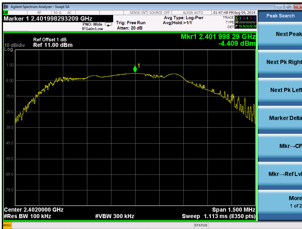
Figure 7: Conducted Spurious Emission, Mode A
