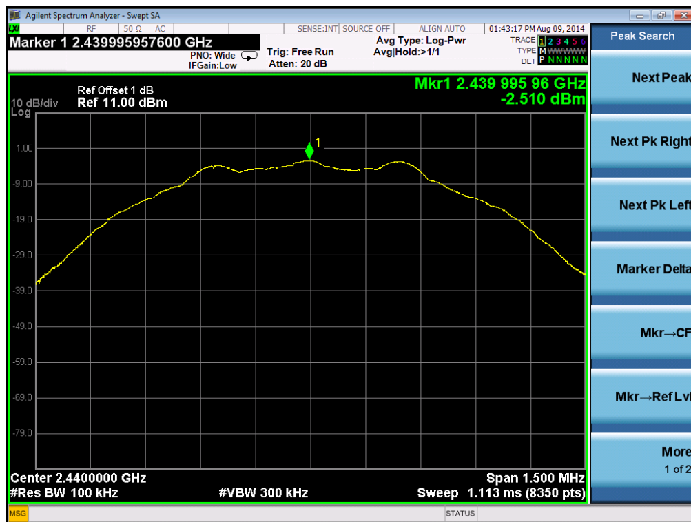
Figure 8: Conducted Spurious Emission, Mode B
