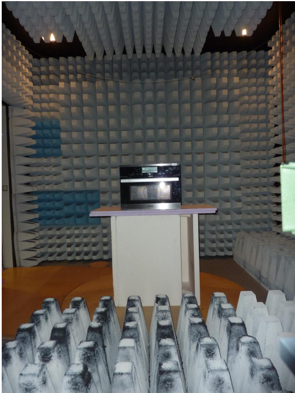
144218_g.JPG: H6700BM, test set-up fully anechoic chamber
