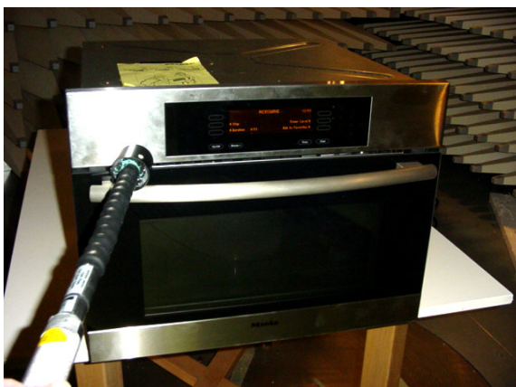
Fig. 1 Radiation leakage test
