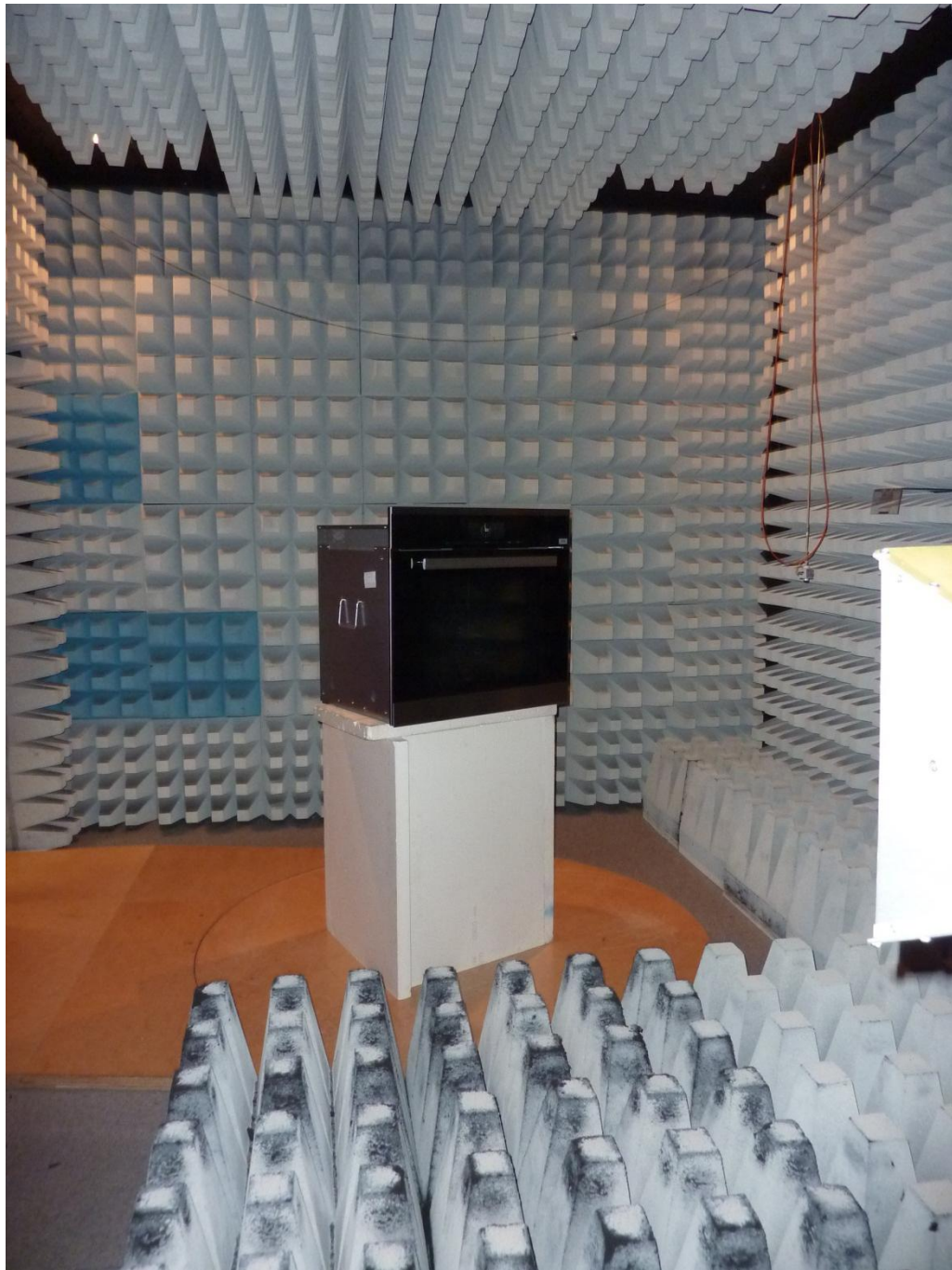
132604_2_2.JPG: EPI7674 inside H6880BP, test set-up fully anechoic chamber
