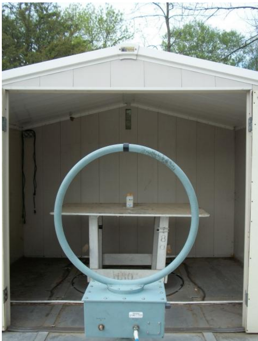
Figure 3.1 Radiated Test Setup
