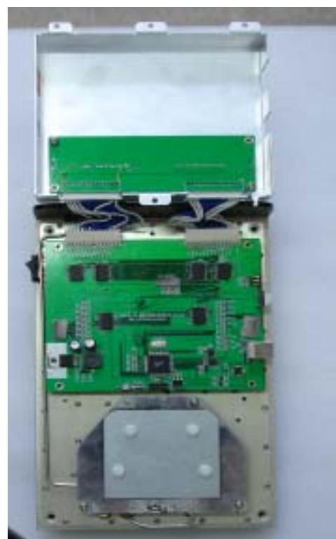
< The Inside of the Repeater >
