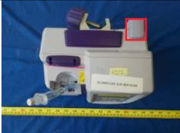
Top position against flat phantom (Ant #1 location) (separation distance – 0cm)
