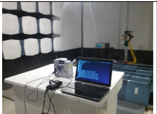
Test setup at 3 meter distance (>1GHz) - Rear
