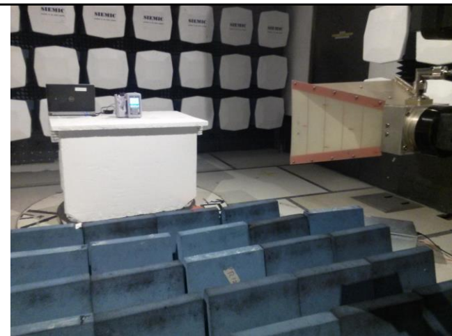
Test setup at 3 meter distance (>1GHz) - Front
