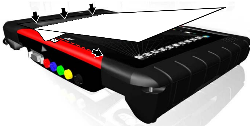
Figure 17-5 Removing rear mask (Tab 1) to apply protector
