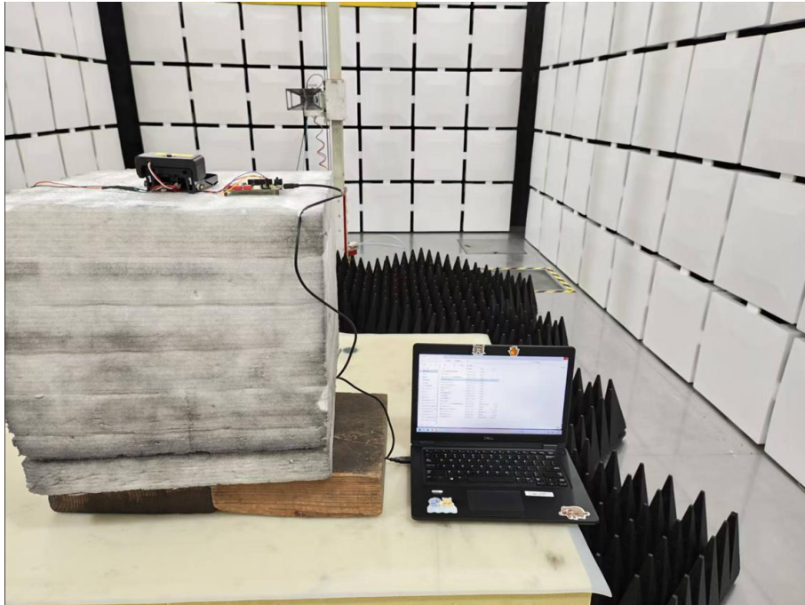
Radiated emission test above 1GHz
