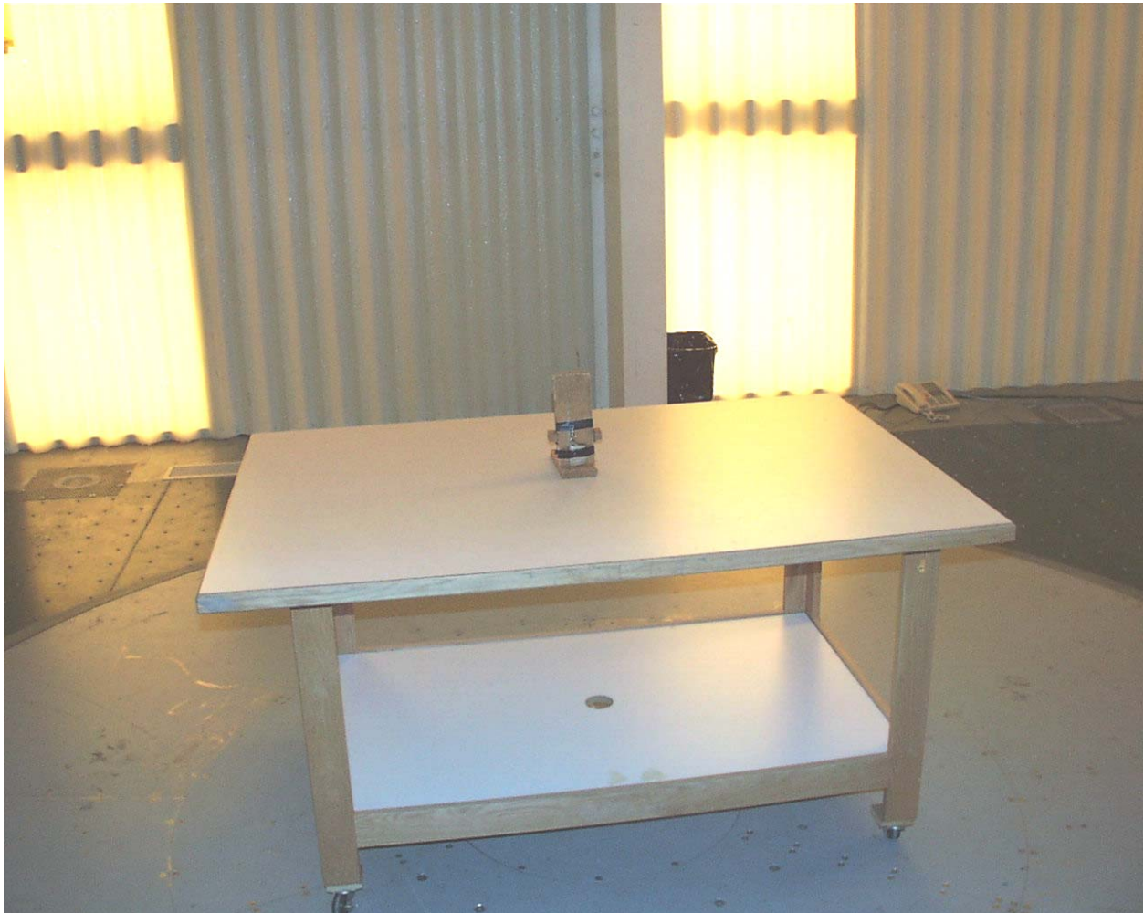
Photograph 1 - View of the Radiated Emission Test Setup (Vertical Alignment)
