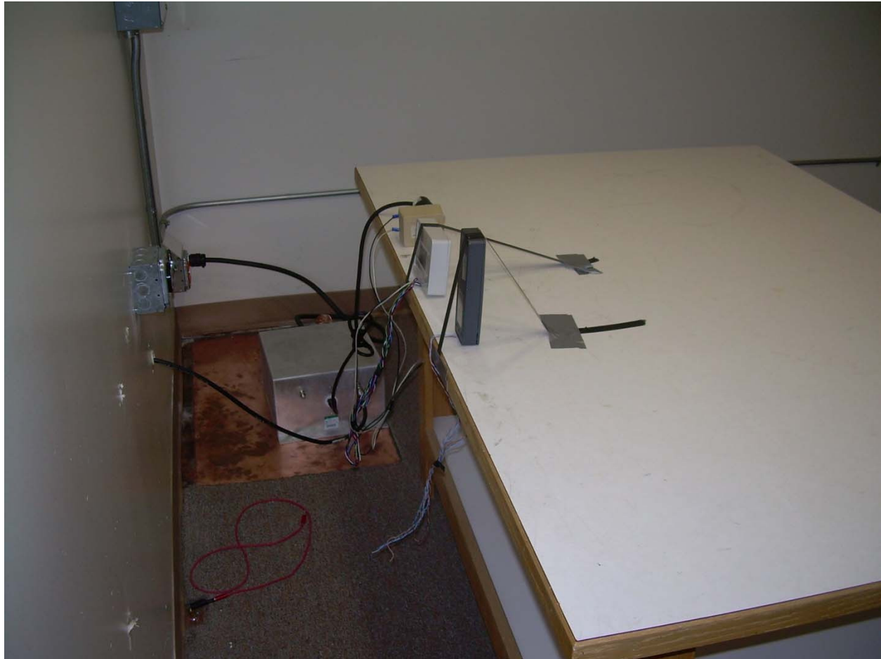
Photograph 4 – Back View Conducted Disturbance Worst Case Configuration
