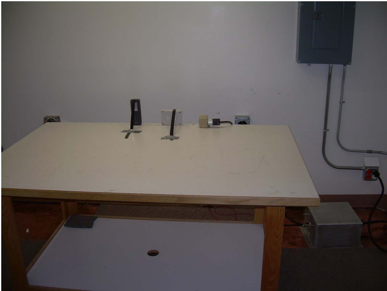
Photograph 3 – Front View Conducted Disturbance Worst Case Configuration
