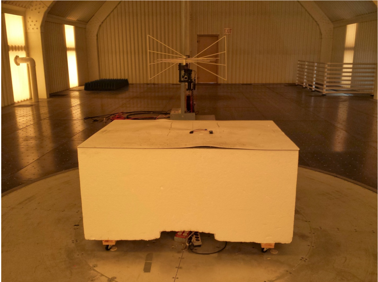
Photograph 1 – Rear View Radiated Disturbance Worst Case Configuration (Flat)
