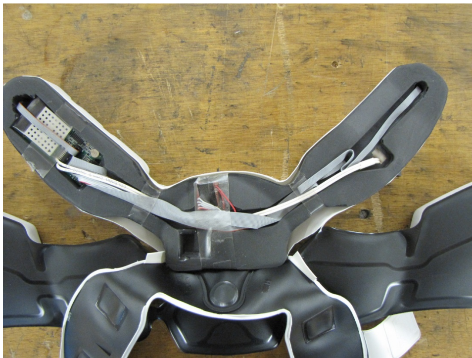
Figure 6 MxEncoder Player Unit and harnesses in final assembly.
