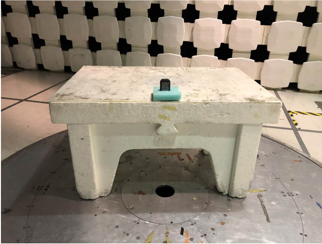
Radiated Emissions Test Setup, 30-1000 MHz
