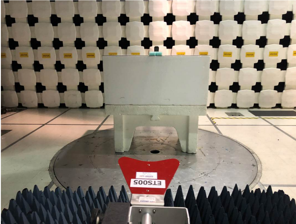
Radiated Emissions Test Setup, 1-13 GHz (Z-axis)
