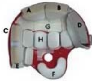
Figure 3: Pad Diagram for Riddell VSR-4 Helmet
