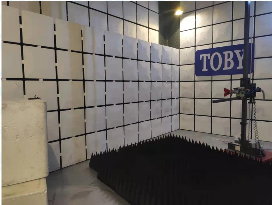
Photo of Setup for Conducted Emission
