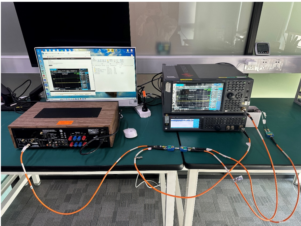
Description: Dynamic Frequency Selection Measurement Test Setup
