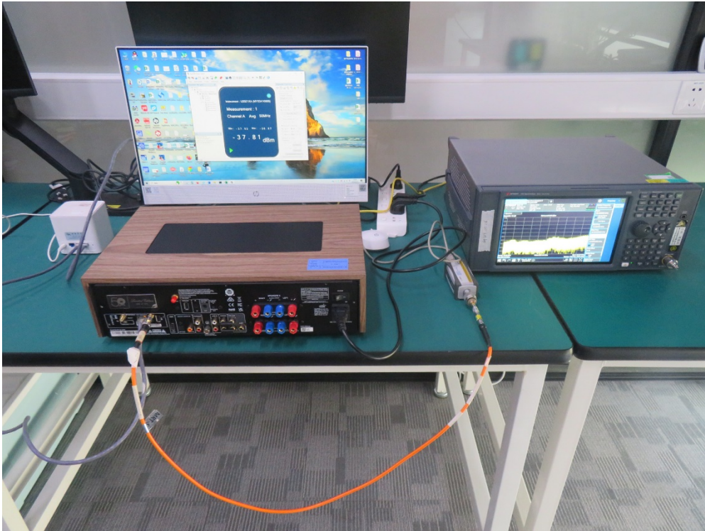
Description: Dynamic Frequency Selection Measurement Test Setup
