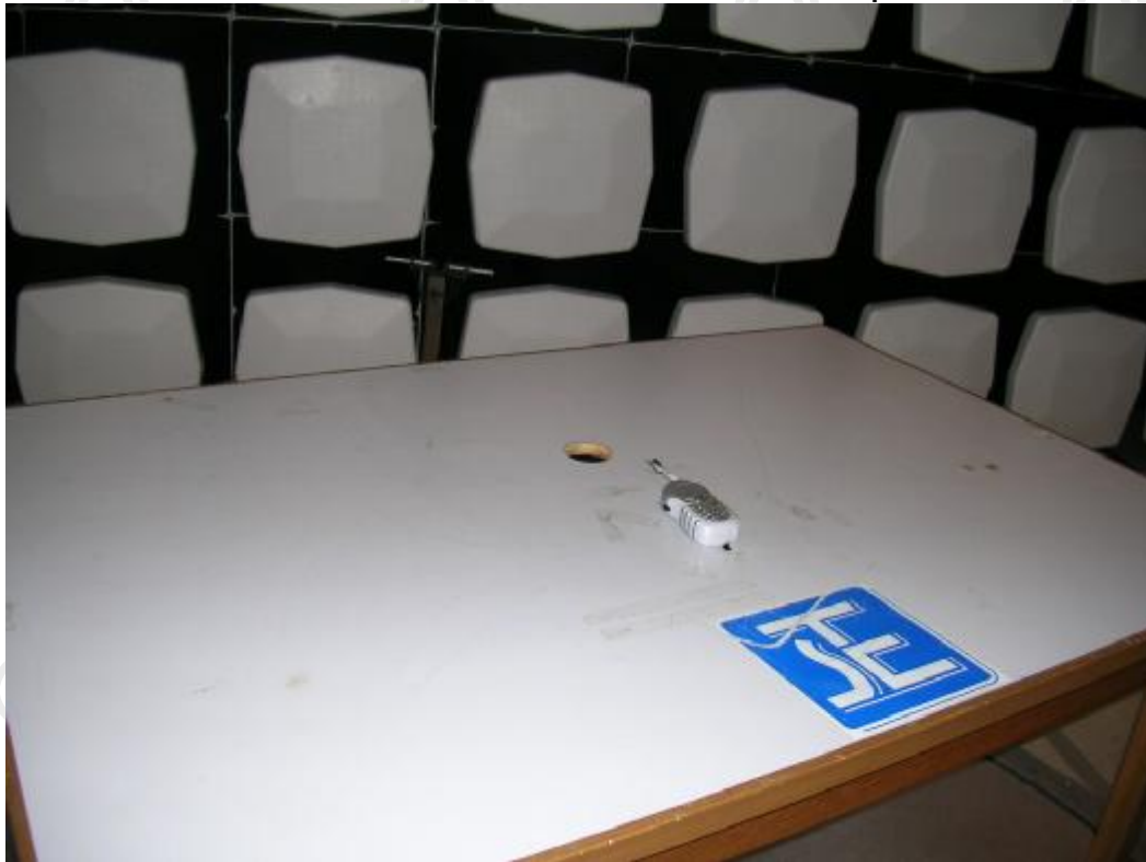
Measurement of Radiated Emission Test Set Up
