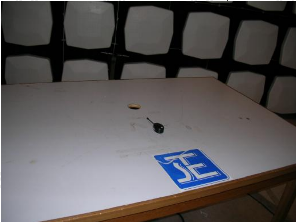
Measurement of Radiated Emission Test Set Up
