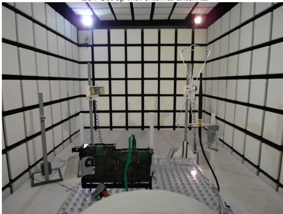
Photo 4 - Spurious Emissions 1 GHz to 12.75 GHz EUT Set-up with external antenna:
