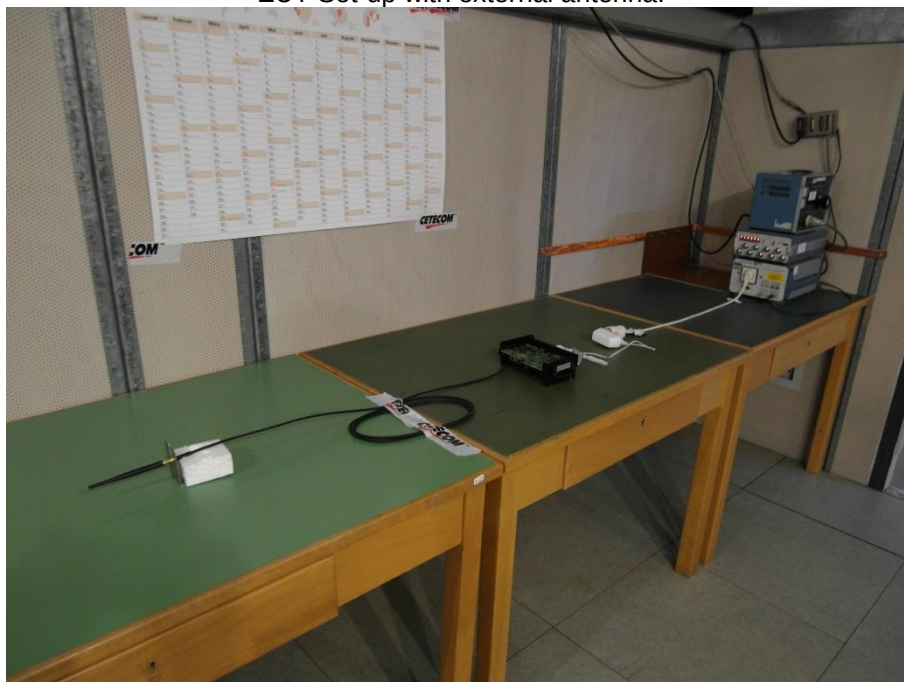
Photo 6 - AC Conducted Emissions EUT Set-up with external antenna:
