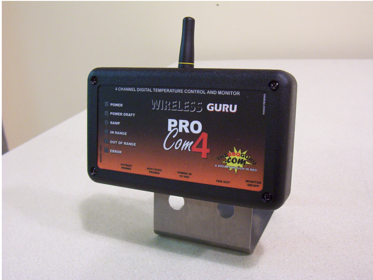
Photo 1 – BBQ Guru Procomm 4 Controller – Front View
