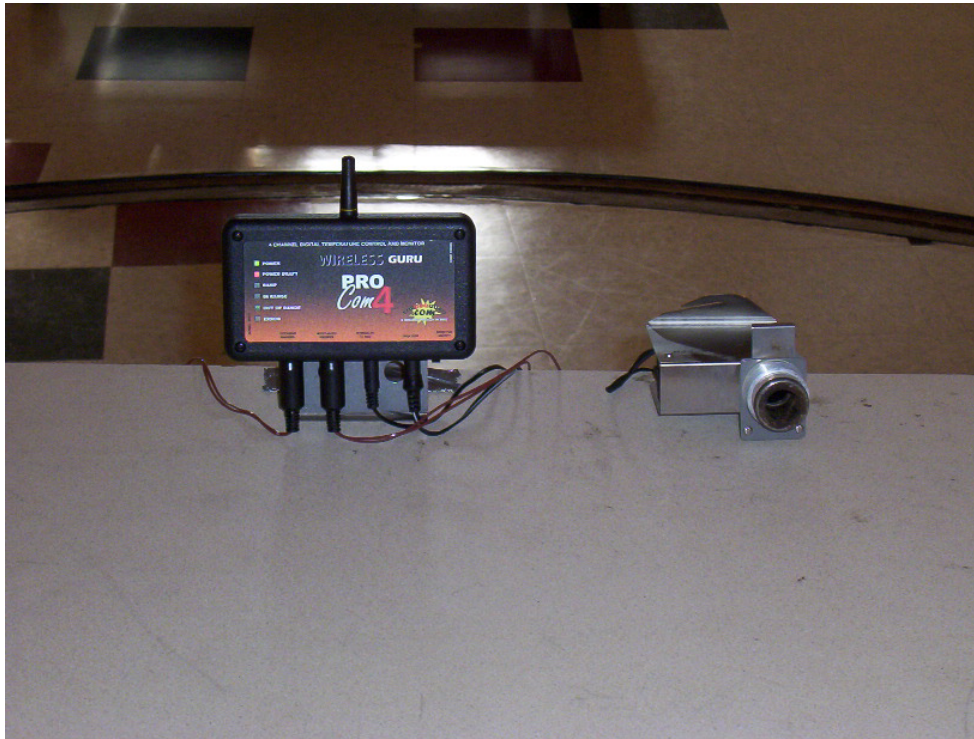
Radiated Emission Test Setup – Front Close up
