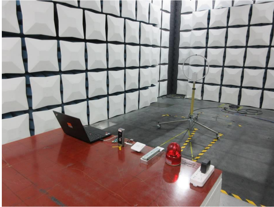
RADIATED RF MEASUREMENT SETUP (9kHz ~ 30 MHz)
