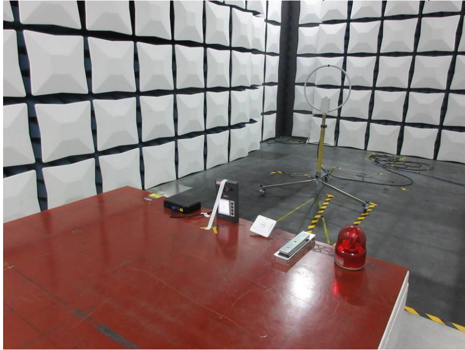
RADIATED RF MEASUREMENT SETUP (9kHz ~ 30 MHz)
