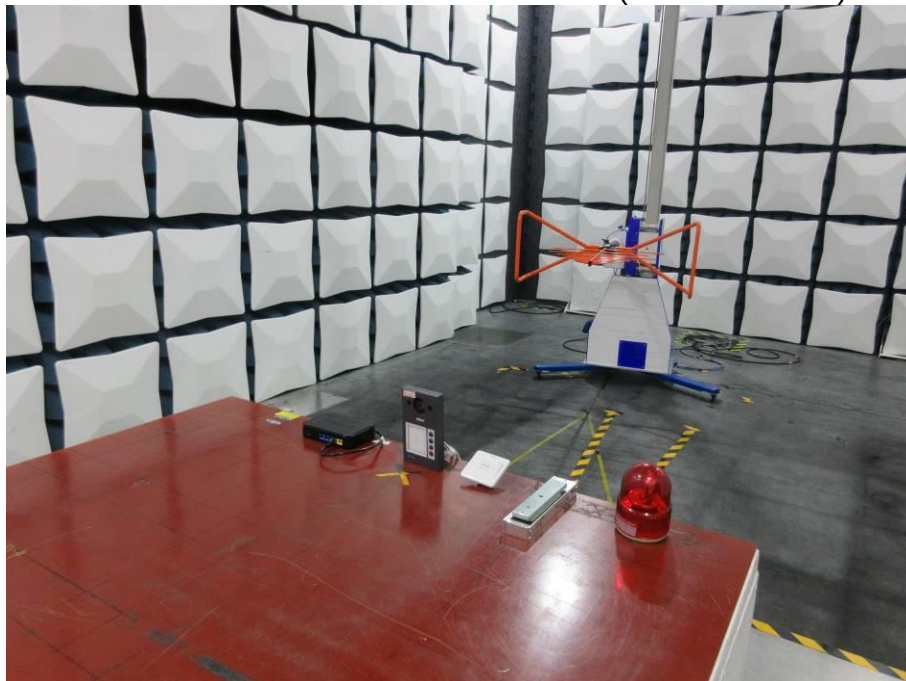
RADIATED RF MEASUREMENT SETUP (30MHz ~ 1 GHz)
