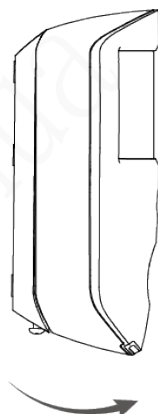
Figure 4-2 Open the PIR-Camera
