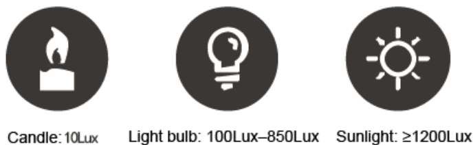
Figure 2-2 Ambient illumination requirement
