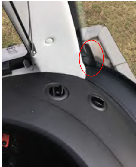
Figure 2-17 Inside installation of Mobile Network Antenna
