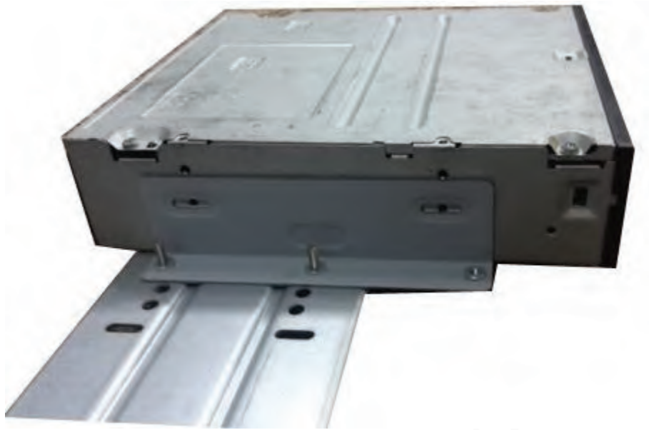
Figure 3-38 Install SATA burner
