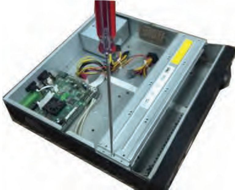
Figure 3-32 Open the top cover
