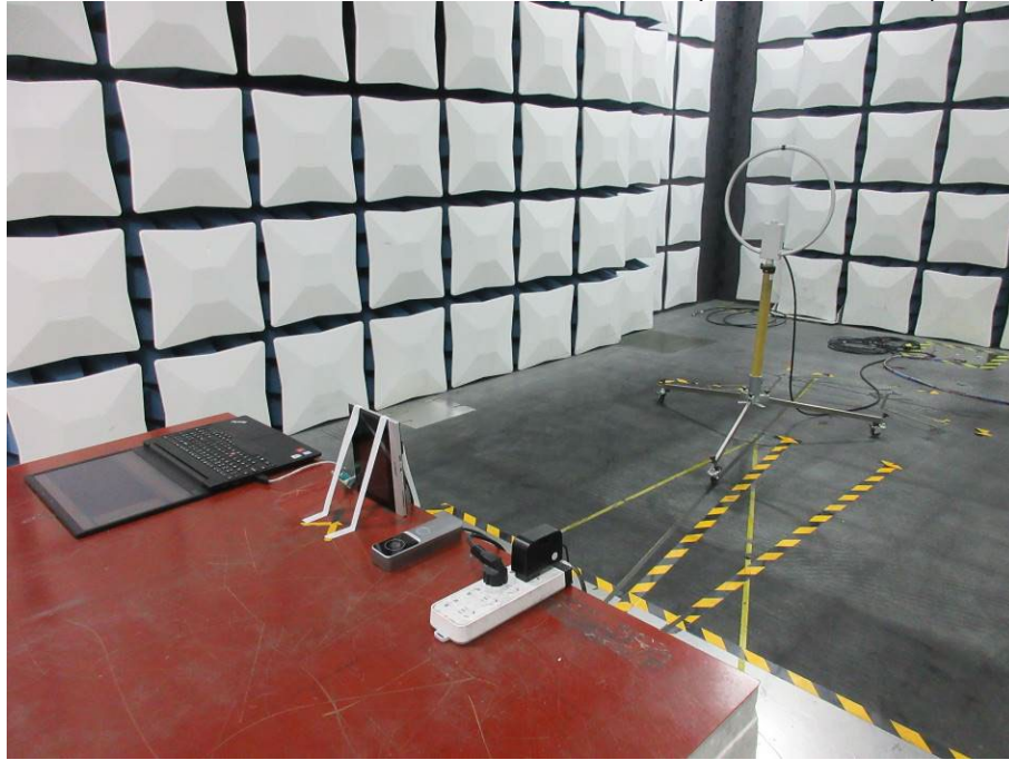
RADIATED RF MEASUREMENT SETUP (9kHz ~ 30 MHz)
