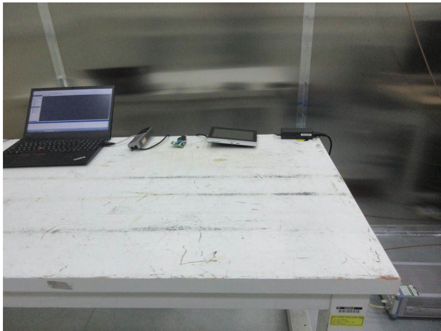
POWERLINE CONDUCTED EMISSIONS MEASUREMENT SETUP
