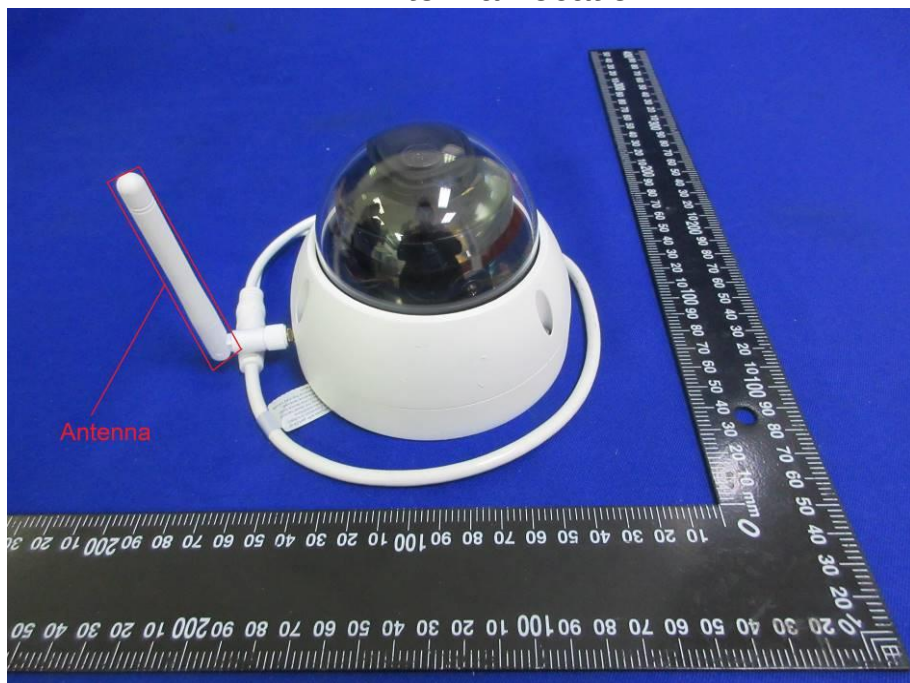
WIFI Antenna Location
