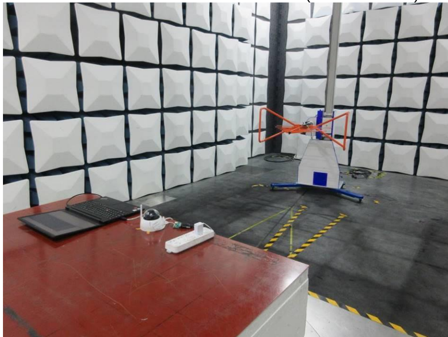
RADIATED RF MEASUREMENT SETUP (30MHz ~ 1 GHz)
