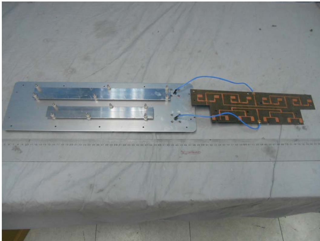
FIGURE 14 AP (M/N: DH-PFM880) ANTENNA (COVER REMOVED)
