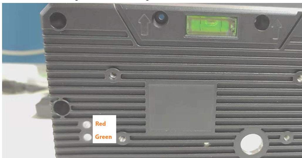
Figure 3-10 Indicator lights on the Radar
