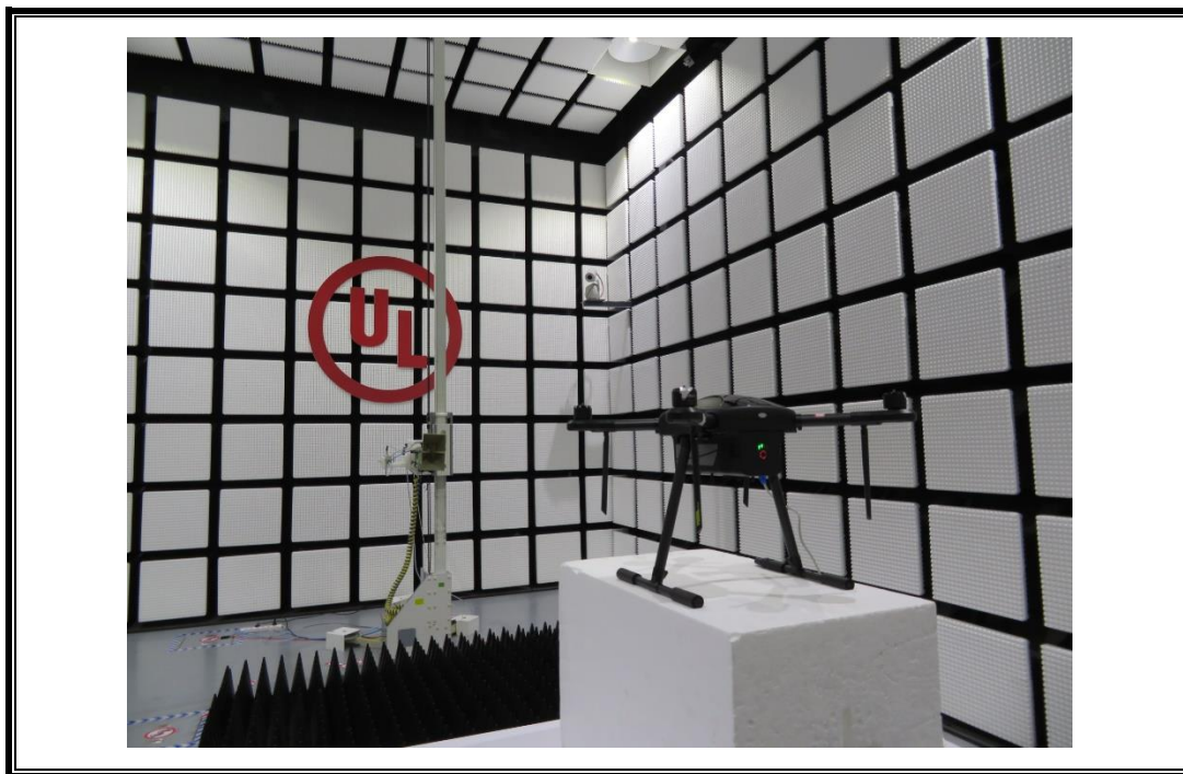
RADIATED RF MEASUREMENT SETUP (ABOVE 1 GHz- Z axis)
