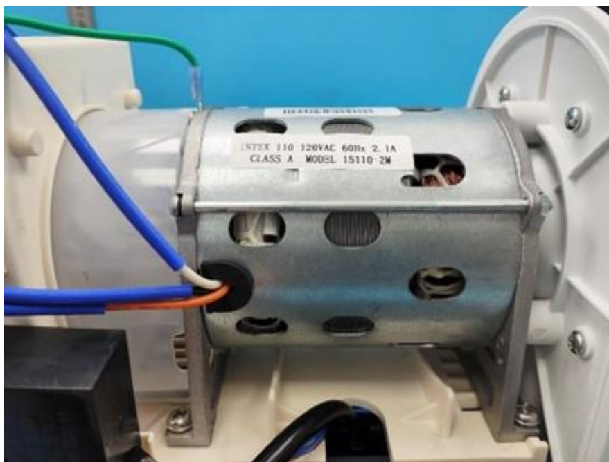
Figure 7: internal view_7 of EUT
