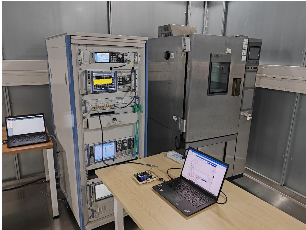
Photograph 2: Set-up for measurement of Conducted Emission
