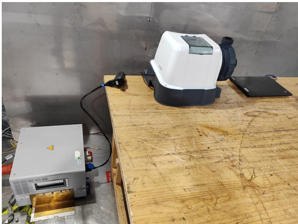
Photograph 2: Set-up for measurement of Conducted Emission
