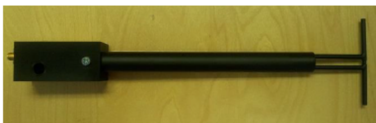
Figure 1 – MVG COMOSAR Validation Dipole
