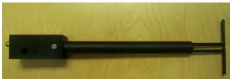
Figure 1 – MVG COMOSAR Validation Dipole
