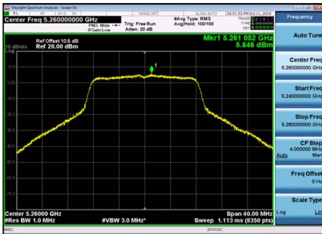
U-NII-2a Power spectral density-802.1 1a(20MHz),5300MHz,Ant1
