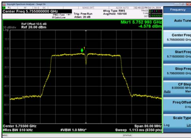
U-NII-3 Power spectral density-802.11 ac(40MHz),5795MHz,Ant1
