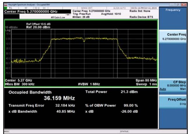
U-NII-2a 26dB Bandwidth-802.11n(40MHz ) ,5310MHz,Ant2
