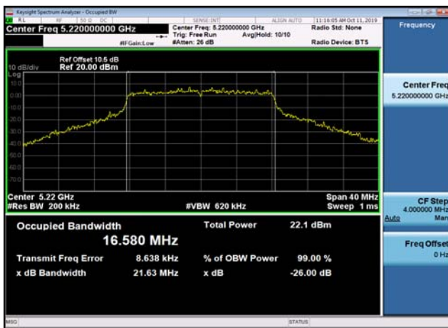
U-NII-1 26dB Bandwidth-802.11a(20MHz) ,5240MHz,Ant1
