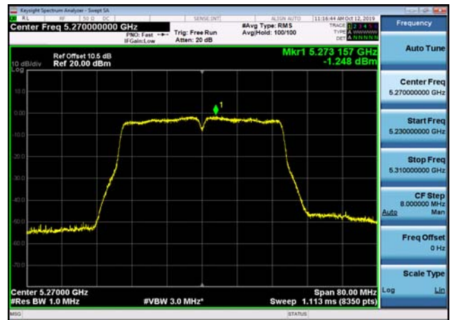
U-NII-2a Power spectral density-802.1 1ac(40MHz),5310MHz,Ant2
