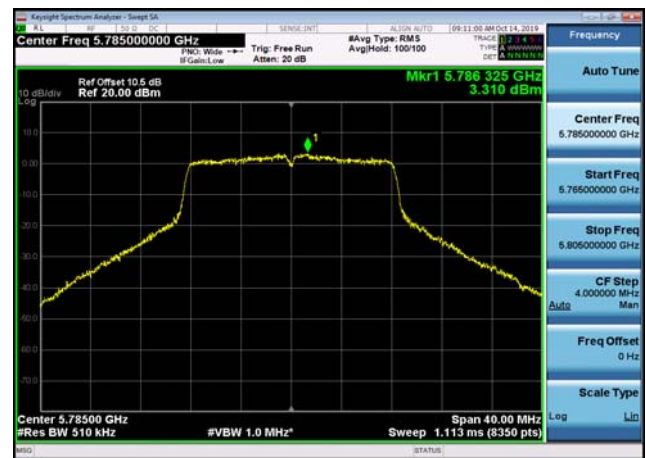
U-NII-3 Power spectral density-802.11 a(20MHz),5785MHz,Ant2
