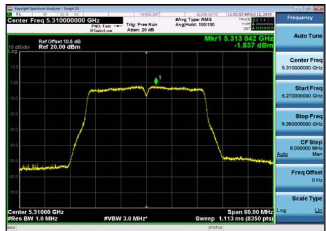
U-NII-2c Power spectral density-802.1 1n(20MHz),5500MHz,Ant2
