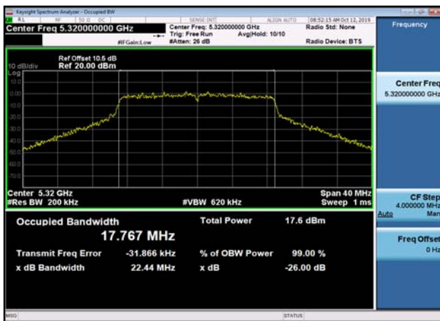
U-NII-2a 26dB Bandwidth-802.11n(40MHz ) ,5270MHz,Ant1
