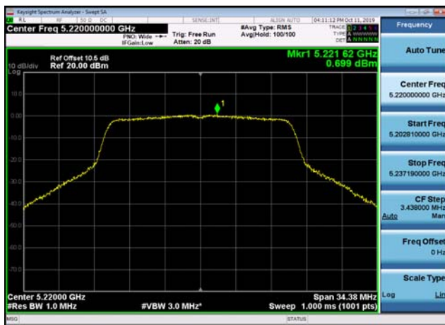
U-NII-1 Power spectral density-802.11 ac(20MHz),5240MHz,Ant1
