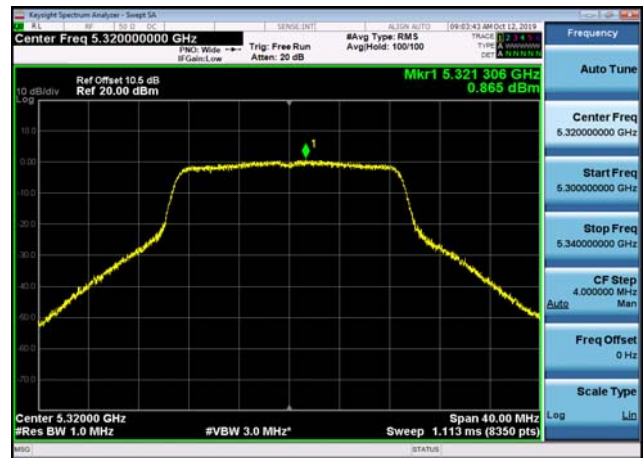
U-NII-2a Power spectral density-802.1 1n(40MHz),5270MHz,Ant2
