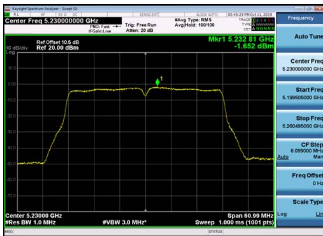
U-NII-2a Power spectral density-802.1 1n(20MHz),5260MHz,Ant1
