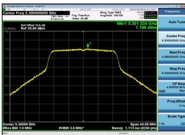
U-NII-2a Power spectral density-802.1 1n(20MHz),5300MHz,Ant1
