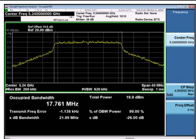
U-NII-1 26dB Bandwidth-802.11n(20MHz) ,5240MHz,Ant2
