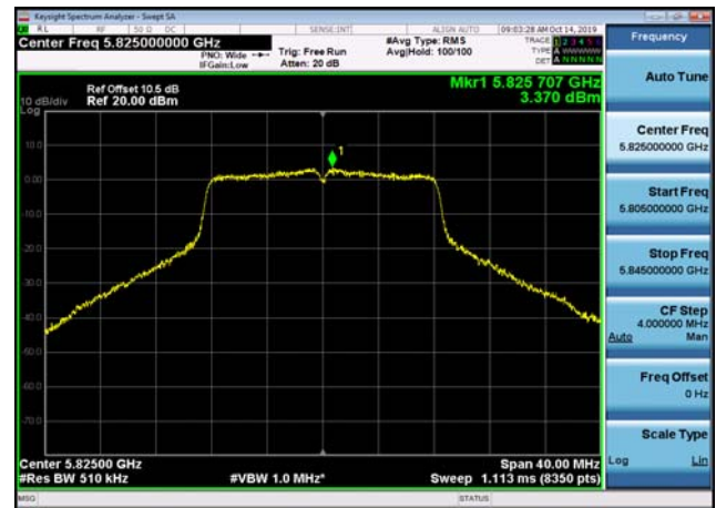
U-NII-3 Power spectral density-802.11 ac(20MHz),5745MHz,Ant2
