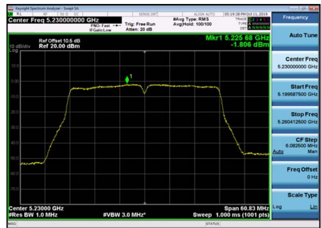
U-NII-1 Power spectral density-802.11 a(20MHz),5180MHz,Ant2
