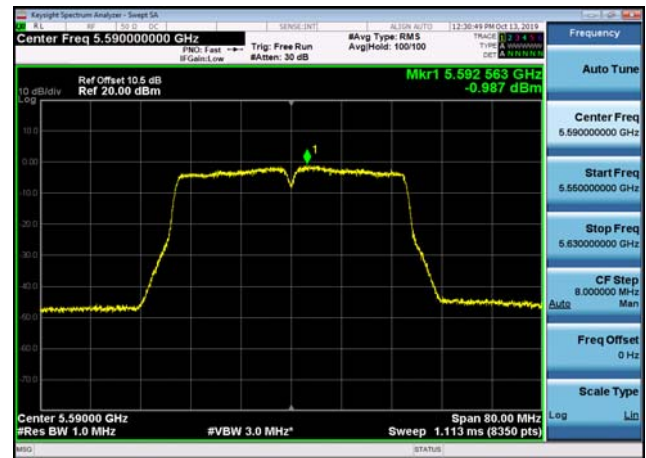
U-NII-2c Power spectral density-802.1 1ac(40MHz),5670MHz,Ant2
