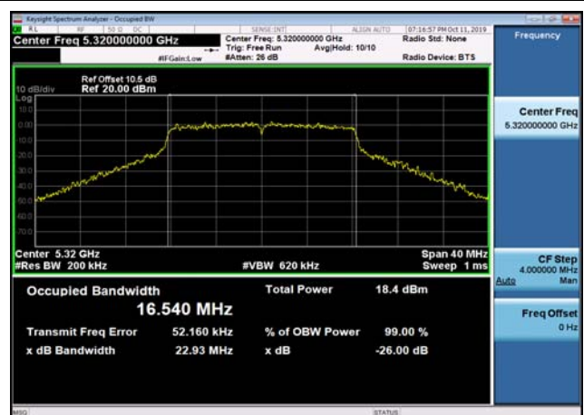
U-NII-2a 26dB Bandwidth-802.11a(20MHz ) ,5320MHz,Ant2
