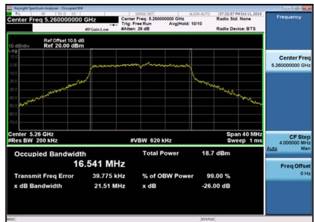
U-NII-2a 26dB Bandwidth-802.11a(20MHz ) ,5300MHz,Ant2
