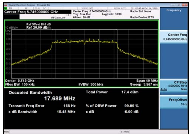
U-NII-3 6dB Bandwidth-802.11ac(20MHz) ,5785MHz,Ant2
