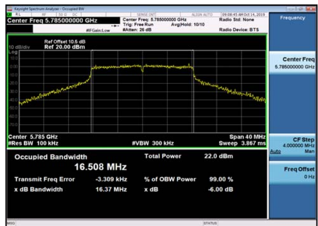
U-NII-3 6dB Bandwidth-802.11a(20MHz) ,5785MHz,Ant2
