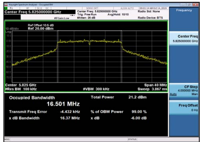
U-NII-3 6dB Bandwidth-802.11ac(20MHz) ,5745MHz,Ant2
