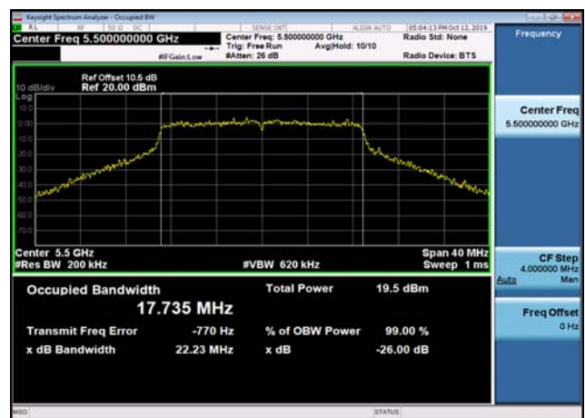
U-NII-2c 26dB Bandwidth-802.11n(20MHz),5500MHz,Ant2
