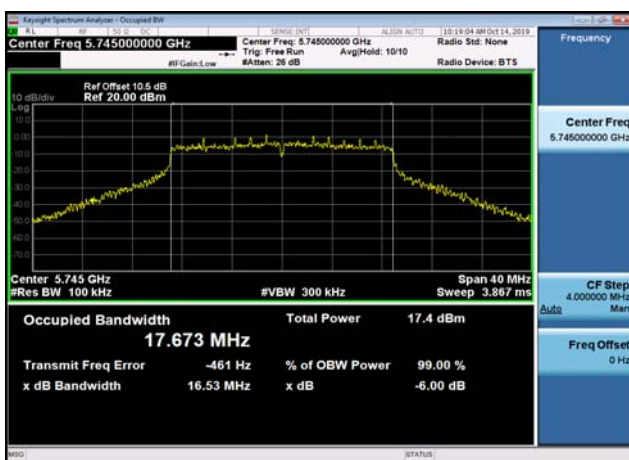
U-NII-3 6dB Bandwidth-802.11n(20MHz),5745MHz,Ant1
