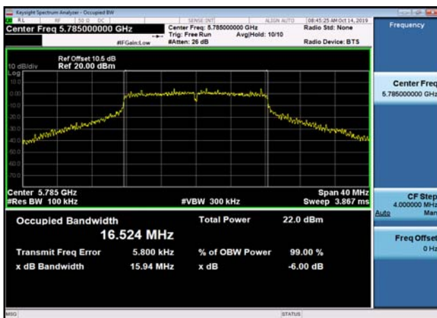
U-NII-3 6dB Bandwidth-802.11a(20MHz) ,5785MHz,Ant1
