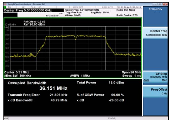
U-NII-2c 26dB Bandwidth-802.11n(20MHz),5500MHz,Ant2
