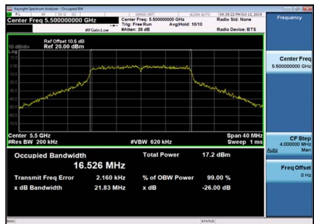
U-NII-2c 26dB Bandwidth-802.11a(20MHz) ,5500MHz,Ant2
