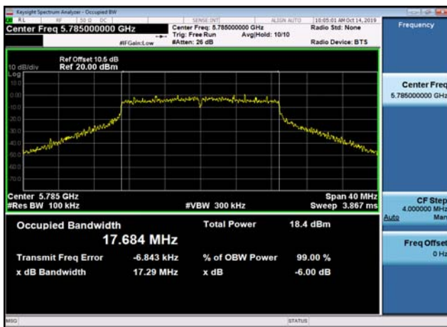
U-NII-3 6dB Bandwidth-802.11n(20MHz) ,5825MHz,Ant1
