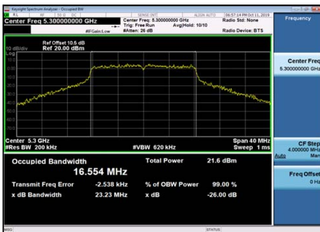
U-NII-2a 26dB Bandwidth-802.11a(20MHz ) ,5320MHz,Ant1
