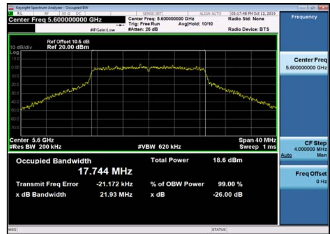
U-NII-2c 26dB Bandwidth-802.11n(20MHz) ,5700MHz,Ant2
