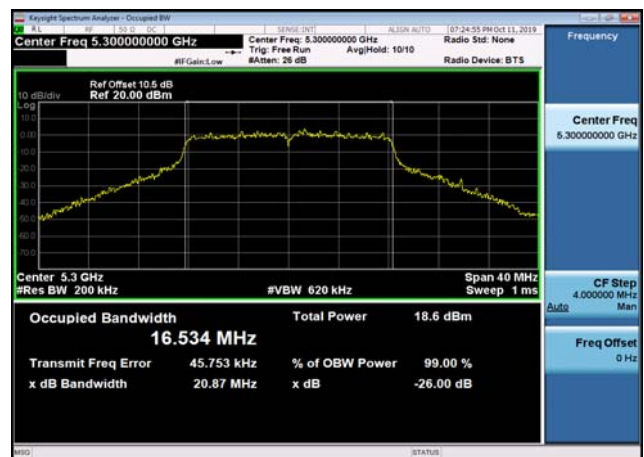
U-NII-2a 26dB Bandwidth-802.11a(20MHz ) ,5320MHz,Ant2
