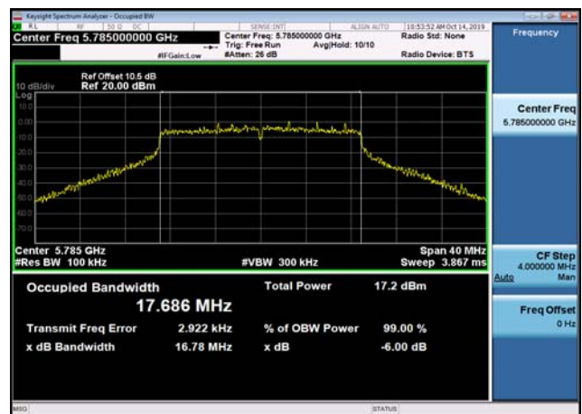
U-NII-3 6dB Bandwidth-802.11ac(20MHz) ,5785MHz,Ant2
