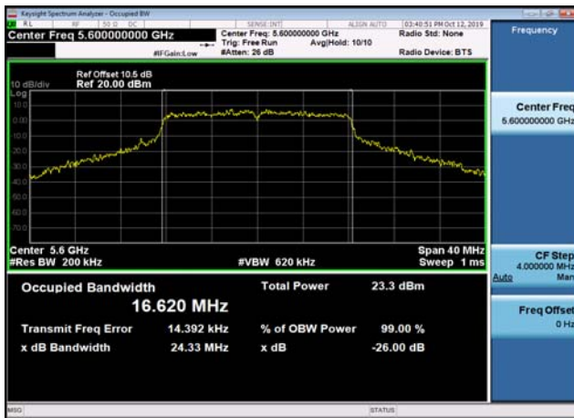
U-NII-2c 26dB Bandwidth-802.11a(20MHz ) ,5700MHz,Ant1
