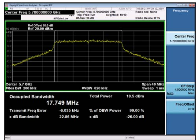
U-NII-2c 26dB Bandwidth-802.11n(40MHz) ,5510MHz,Ant2
