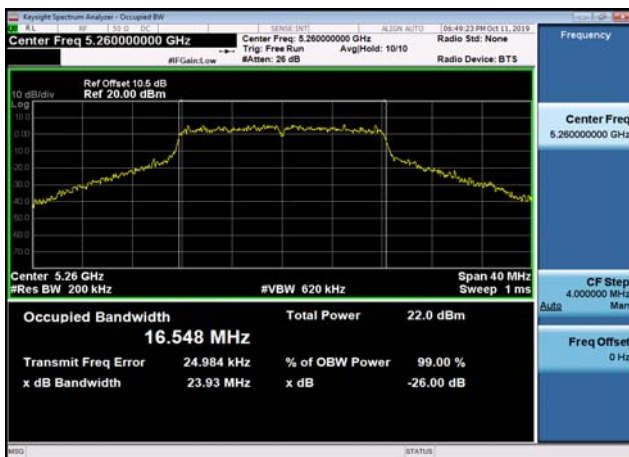
U-NII-2a 26dB Bandwidth-802.11a(20MHz ) ,5300MHz,Ant1
