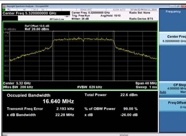
U-NII-2a 26dB Bandwidth-802.11a(20MHz ) ,5320MHz,Ant1
