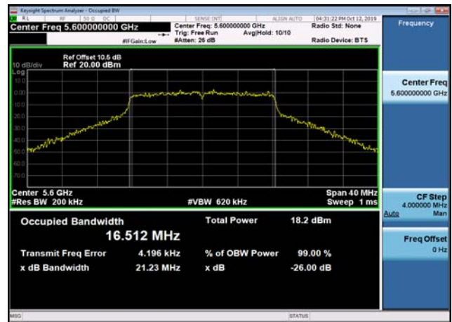
U-NII-2c 26dB Bandwidth-802.11a(20MHz ) ,5700MHz,Ant2
