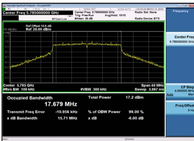
U-NII-3 6dB Bandwidth-802.11ac(20MHz) ,5785MHz,Ant1
