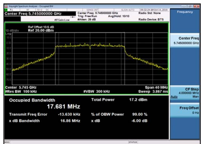
U-NII-3 6dB Bandwidth-802.11n(20MHz),5745MHz,Ant2
