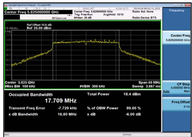
U-NII-3 6dB Bandwidth-802.11n(40MHz) ,5755MHz,Ant2
