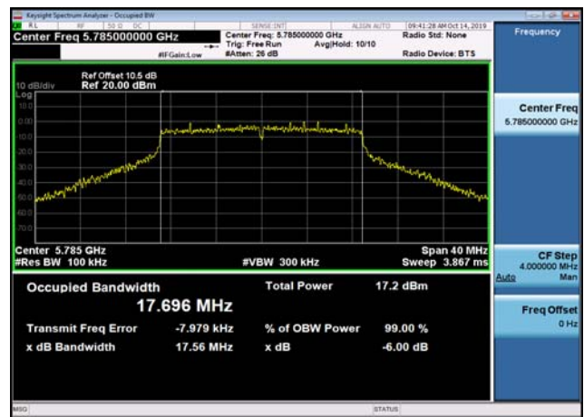
U-NII-3 6dB Bandwidth-802.11n(20MHz) ,5825MHz,Ant2
