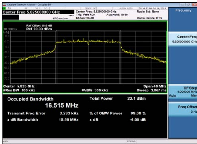
U-NII-3 6dB Bandwidth-802.11ac(20MHz) ,5745MHz,Ant1
