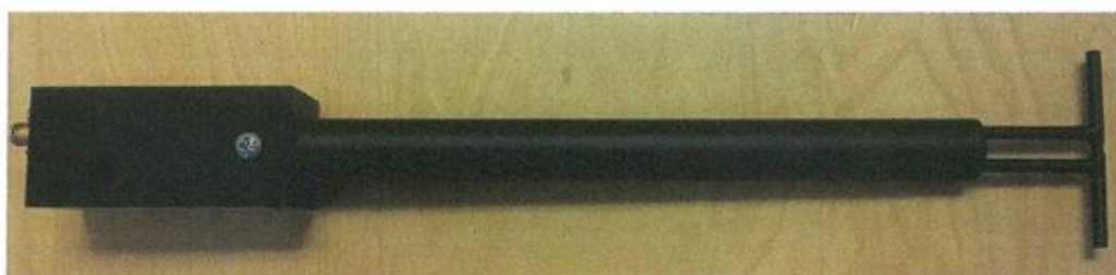
Figure 1 – MVG COMOSAR Validation Dipole
