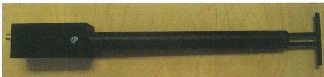
Figure 1 – MVG COMOSAR Validation Dipole
